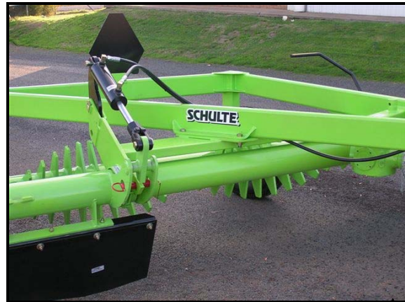
Special Features on the Schulte SRW1000 Adjustable Barrel angle from 18" to 22"
